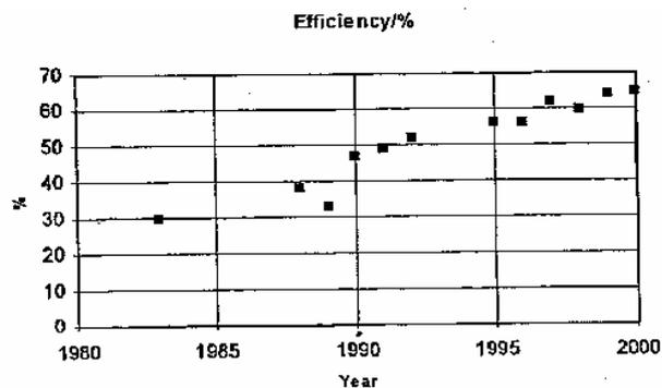
Fig.3.3 Trend of DC-RF Conversion Efficiency of TWTA [17]
