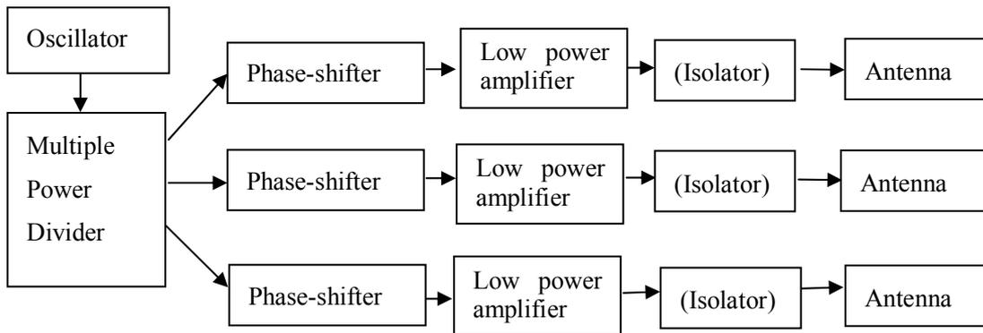
Fig. 6.4 Implementation of microwave transmission with phase-shifters and low power amplifiers for high precision control of microwave beam direction without grating lobes
