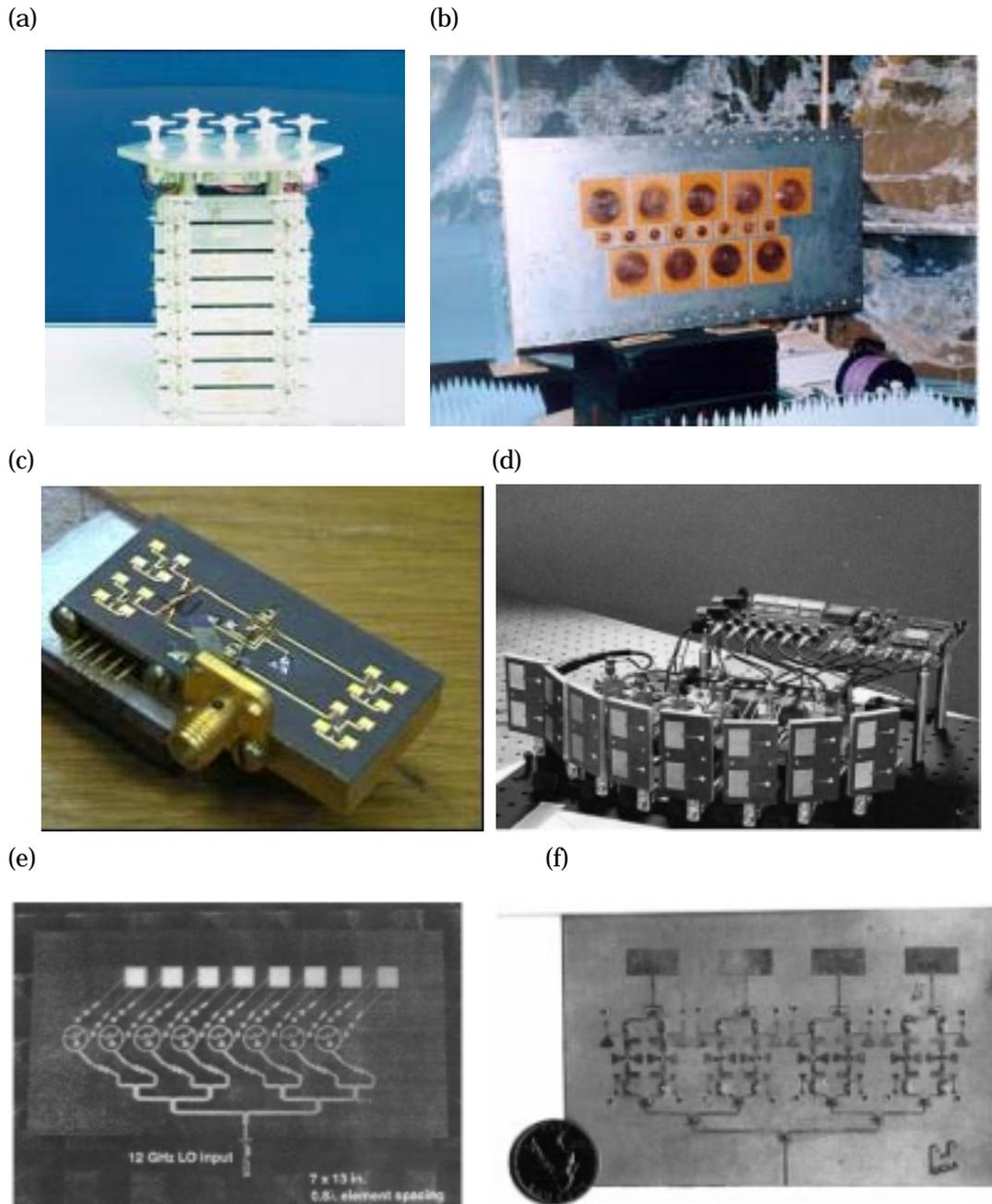
Fig.4.2 Various Retrodirective Array with Phase Conjugate Circuits Developed in
